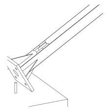
Figure 7 Lifting the Pole into Position
